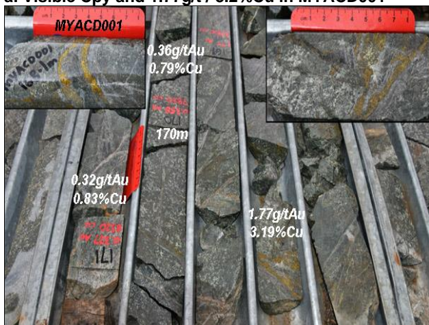
Figure 12. 3d Mag Schematic Cross-section of Myall, and Encouraging Mineralisation and Specimens in NACD158 a. Visible Cpy and 1.77g/t / 3.2%Cu in MYACD001 b. Encouraging Mineralisation and Specimens in NACD158
